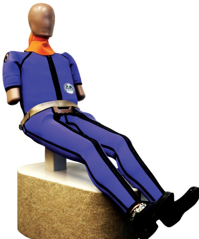
The original WorldSID crash test dummy was developed over the course of six years by an international team. Image courtesy of WorldSID.
