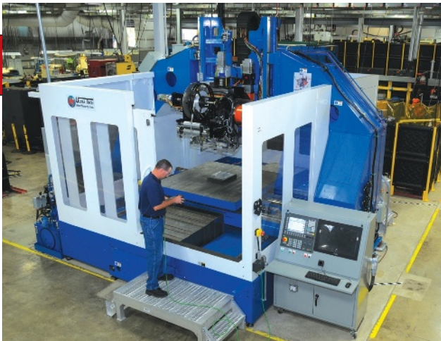
SonicLayer 7200 Ultrasonic Additive Manufacturing (UAM) system from Fabrisonic. Ultrasonic welding process creates a solid-state bond between layers of similar or dissimilar metals. Image courtesy of Fabrisonic.
